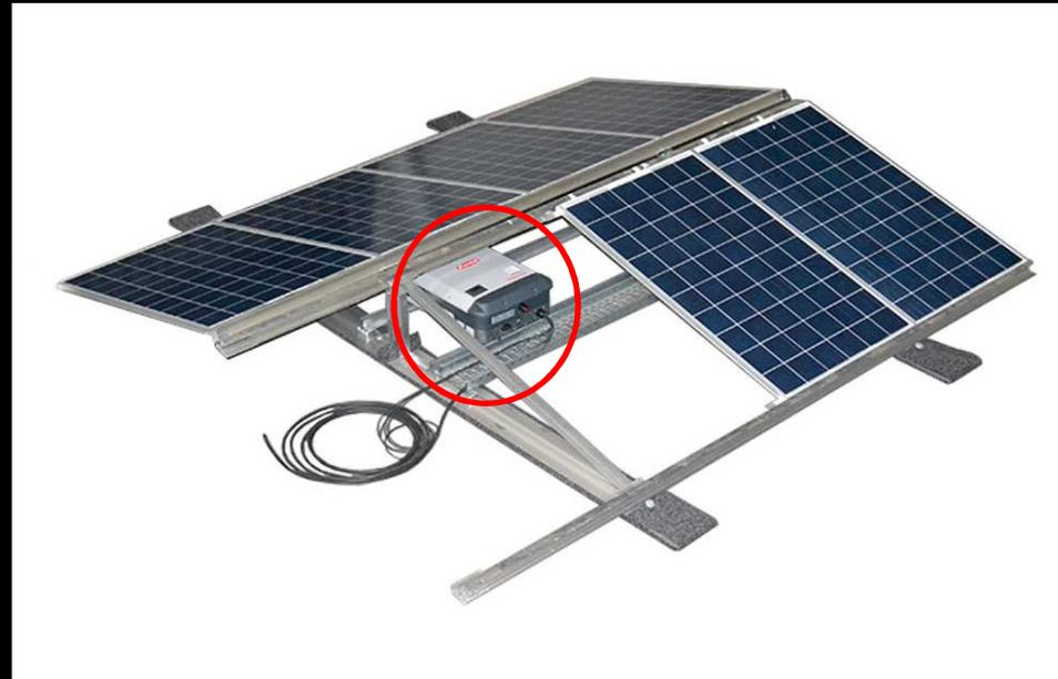
The SOL-50 flat roof mounting system DUO FLEX offers the option of decentralized inverter installation in the system. Thus the inverter is secured against weather conditions but nevertheless aerated. Thanks to the decentralized inverter concept only short cables are necessary. The inverter will be quickly and safely installed on an inverter bracket which guarantees accessibility.
