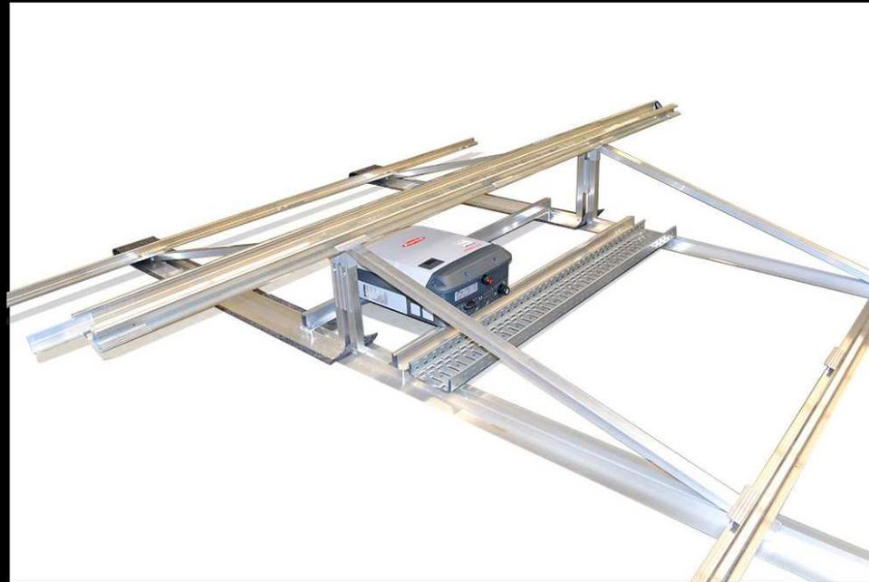
A cage for more security. With the SOL-50 mounting system the module has no carrying role. The mounting system carries itself and thus keeps away the loads from the solar module. There the triangle consoles and the horizontal profiles exclusively form the group.
